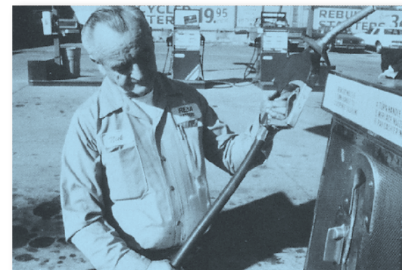
Inspect hose cover for cracks or cuts.
