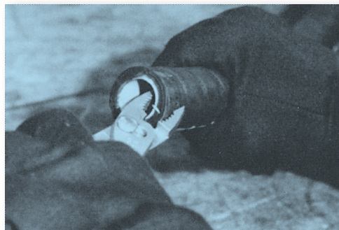
Helix wire being bent into the inner surface of the hose tube.
